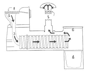
The human excrement falls down a vertical chute (2) and into one end of a specially designed helical screw conveyor (3). Every time the toilet lid (1) is lifted, a mechanism rotates the conveyor. With each rotation the human excrement slowly moves along, taking approximately twenty
