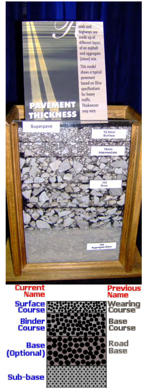
Fig. B.1 Construction Makeup of Typical Road
